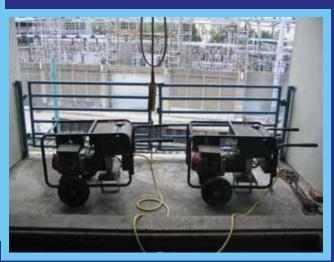
Gasoline generators, submersible pumps, and oxygen concentrators
